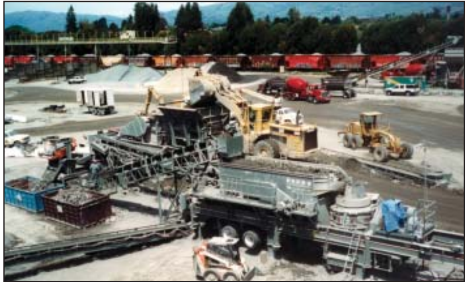
Secondary system consists of a 7' x 20' horizontal screen, and a TelSmith 57 SBS (Silver Bullet Series) cone crusher.
