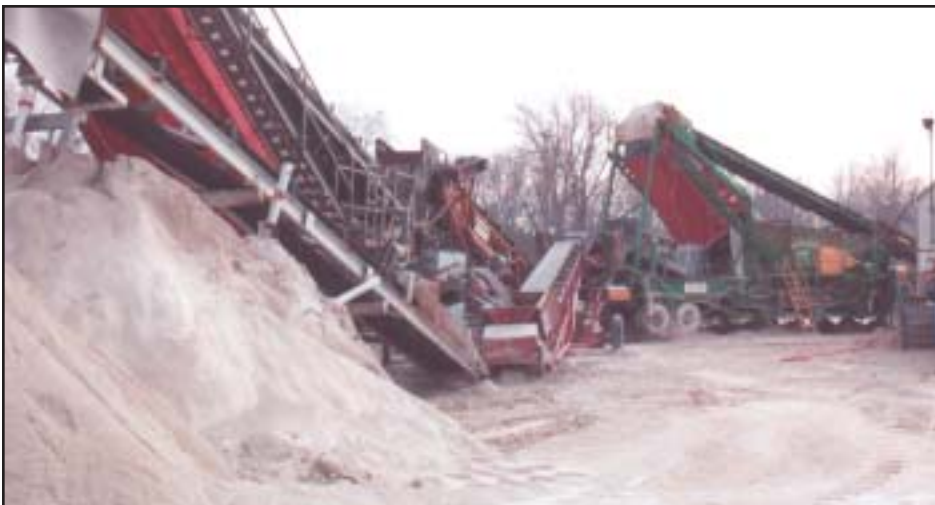
PEP Super Series III plant feeding a PEP PTSC plant at Franklin Aggregates.
