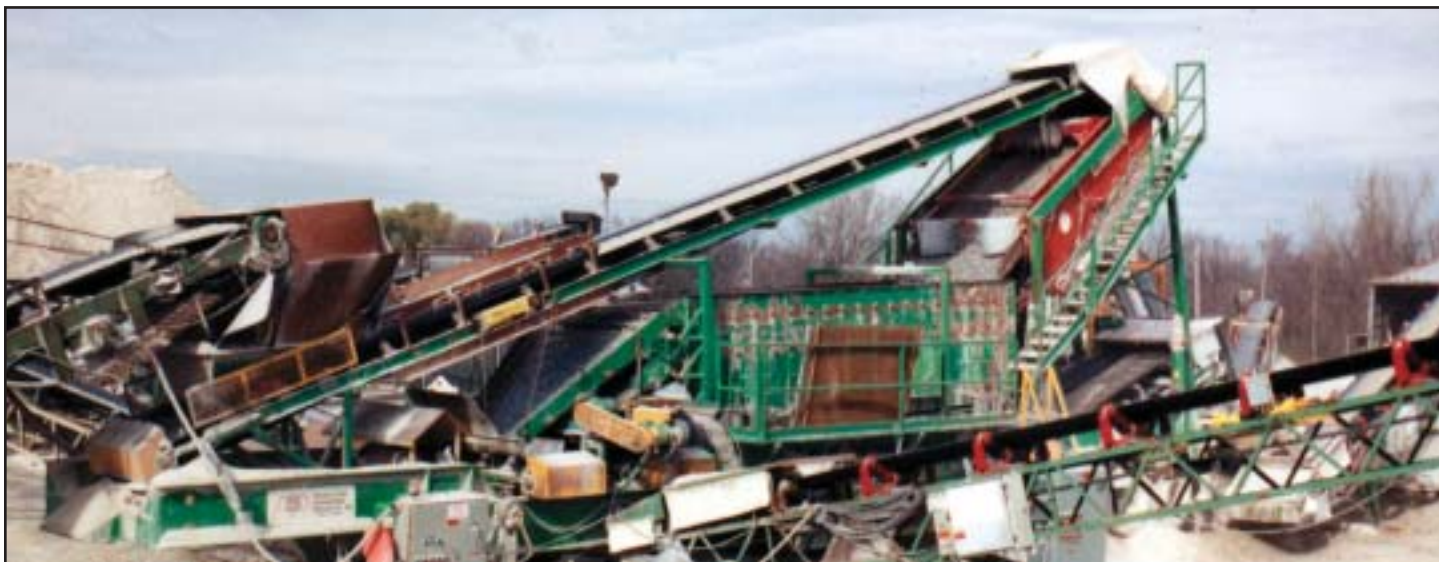
PEP's Super Series III high frequency screening plant hard at work at Franklin Aggregates.
